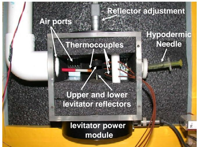
Fig. 1. Oscillation levitator and environmental chamber. The grey background material surrounding labeled components is foam insulation.
