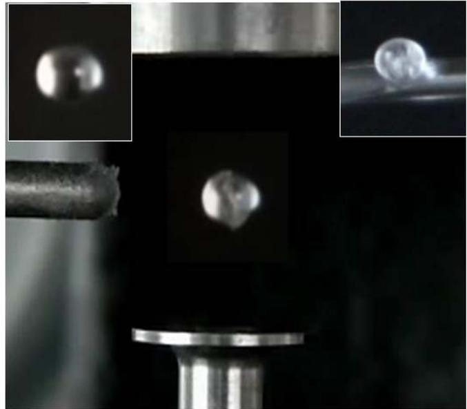
Fig. 7. A nucleation event during the oscillation experiments. The upper left inset shows the drop before freezing, and the upper right inset shows the frozen drop resting on the hypodermic needle after capture.
