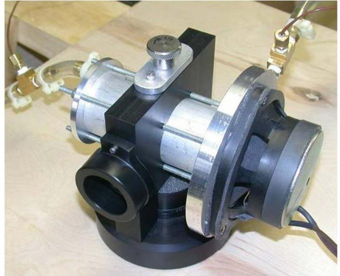
Fig. 4. Resonator as constructed. Cold air flows in, and out, through the plastic tubing. The video camera attaches to the open port on the lower left. The thumb-knob on top controls the levitator reflector height. The loudspeaker used to insonify the chamber is on the right.
