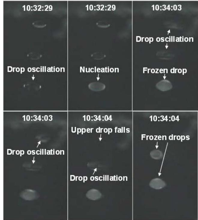
Fig. 9. A sequence of two drops freezing about 1.5-minutes apart due to oscillation in the levitator. The top of each image is up.
