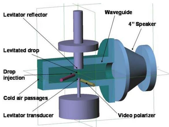
Fig.3. Resonator as designed [20].
