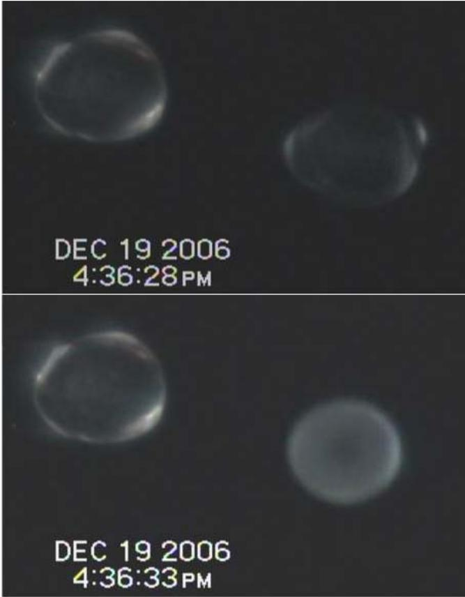
Fig. 8. The drops in the top frame are vigorously oscillating as indicated by their shape. In the bottom frame, the right drop has nucleated, but the left drop did not freeze. The top of each image is up.
