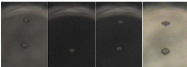
Fig. 11. The bottom drop froze without acoustic stimulation shortly after being injected into the resonator. The upper drop nucleated during the acoustic pulse. The top of each image is up, and the time sequence is left to right.
