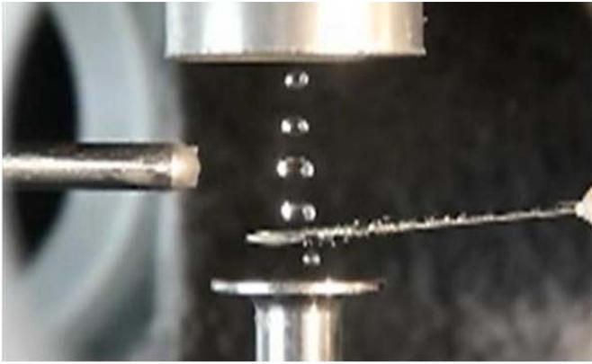
Fig. 5. Multiple drops were often initially levitated because water droplets injected into the chamber were captured by several levitator acoustic nodes. Drops were removed by attaching them to the hypodermic needle.
