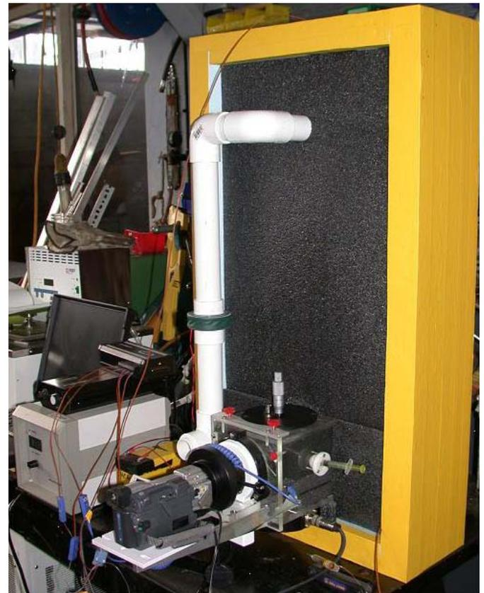
Fig. 2. Air is chilled by a heat exchanger within the insulation-filled box. The video camera attaches to a plastic cover on the front of the levitation chamber.
